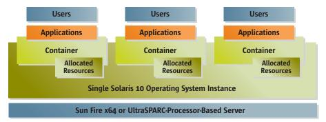
Figure 1. Multiple Solaris Containers on a single Solaris 10 OS instance.
